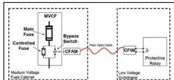
Figure 7: Controllable Fuse Diagram
