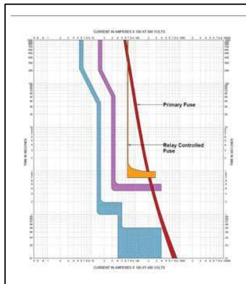
Figure 8b: Time Current Curves of Controlled Fuse with 200 ms delay
