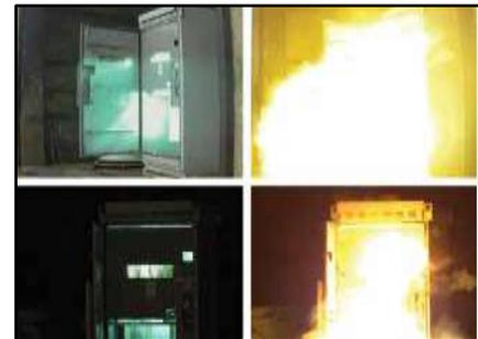
Figure 2. Reach of arc flash with E-Rated Fuse (l) and 5 cycle opening (r)
