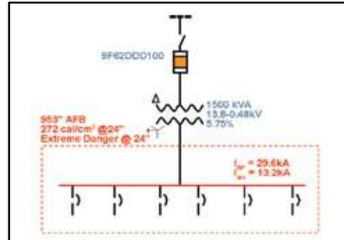
Figure 4: Switchgear with no main fed by 1500KVA Transformer. Short circuit protection for switchgear bus is provided by primary fuse.
