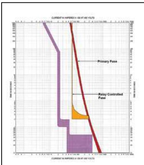
Figure 9b: Time Current Curves of Controlled Fuse with 700 ms delay
