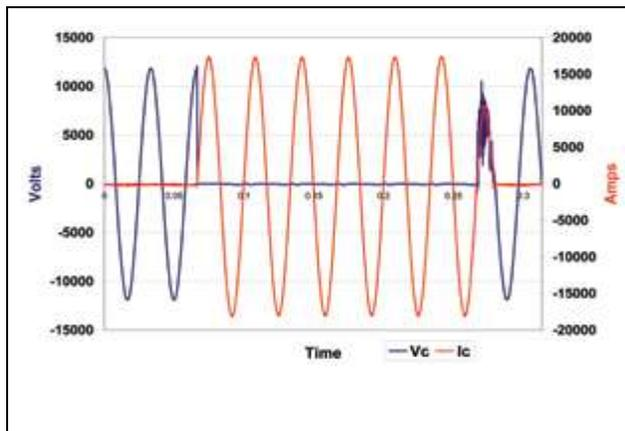
Figure 3a: Bolted Fault test with 5 cycle clearing time
