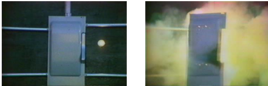
Figure 2-2 10kAIR OCPD interrupting 25kA.
