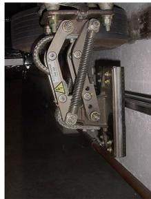
Current collector devices are used by Metro to collect the energy from the third rail to energize the Electrical Multiple Unit installed in the trailers.
