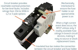
Overloads are the most common overcurrent condition and the MFCP's innovative combination branch circuit protection provides resettable overload protection up to 2 times the circuit rating while still providing true class CC and J protection for your critical loads on high current faults. MFCP branch circuit protection devices can be ordered to replace or add new branch circuits within a panel.
