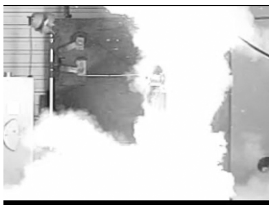
Fig. 11. Side view of Test 69 with enclosure O at 10kA Test
