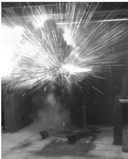
Fig. 8 Video capture after enclosure failed to contain arc flash hazards
