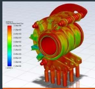
Heating simulation within a slip ring
